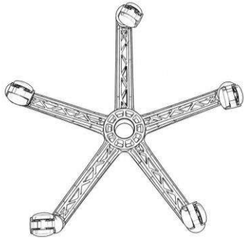
Step 1: Fit castors into base
